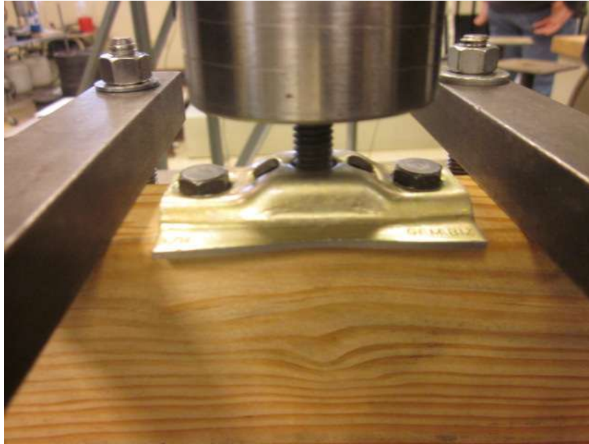
Photo No. 3 Typical Fastener Withdrawal Test Setup Detail
