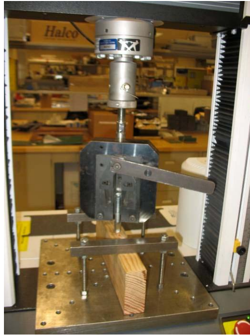
Photo No. 3 Fastener Withdrawal Test Setup
