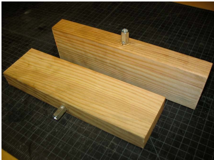
Photo No. 2 Depiction of Typical Pretest Condition Test Specimens with Embedded Hanger Screw (Tangential Face Embedment Specimen [Front] Radial Face Embedment Specimen [Rear])
