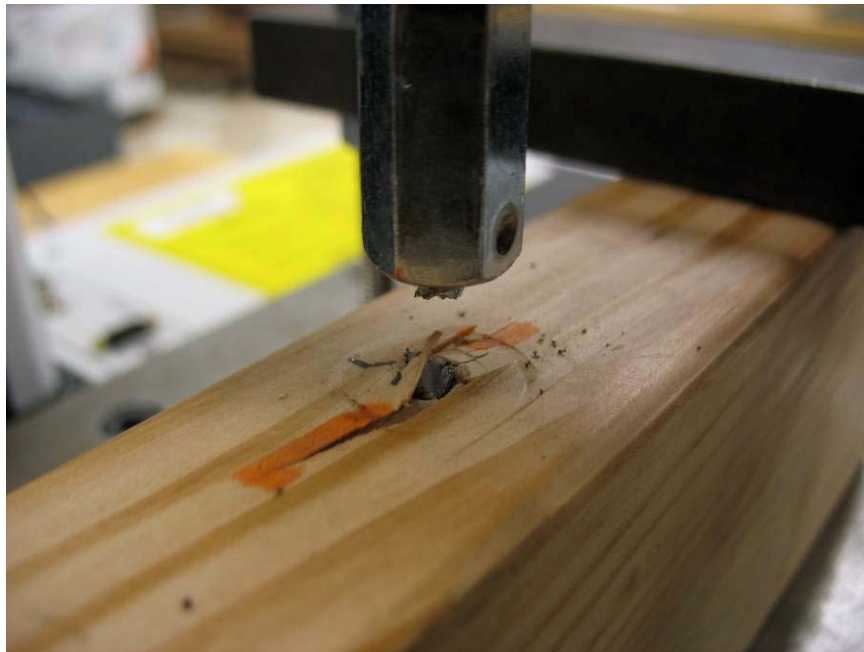
Photo No. 6 Typical Fastener Rupture Failure Mode Detail (Tangential Face Fastener Embedment Depicted)
