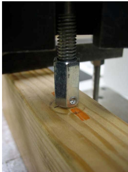
Photo No. 4 Typical Pretest Condition Fastener Embedment Detail
