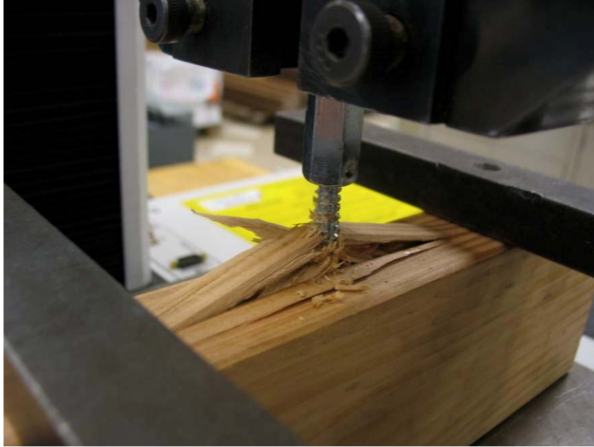
Photo No. 5 Typical Fastener Withdrawal Failure Mode Detail (Radial Face Fastener Embedment Depicted)
